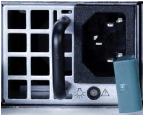
Figure 18. Removing a PSU from the chassis
